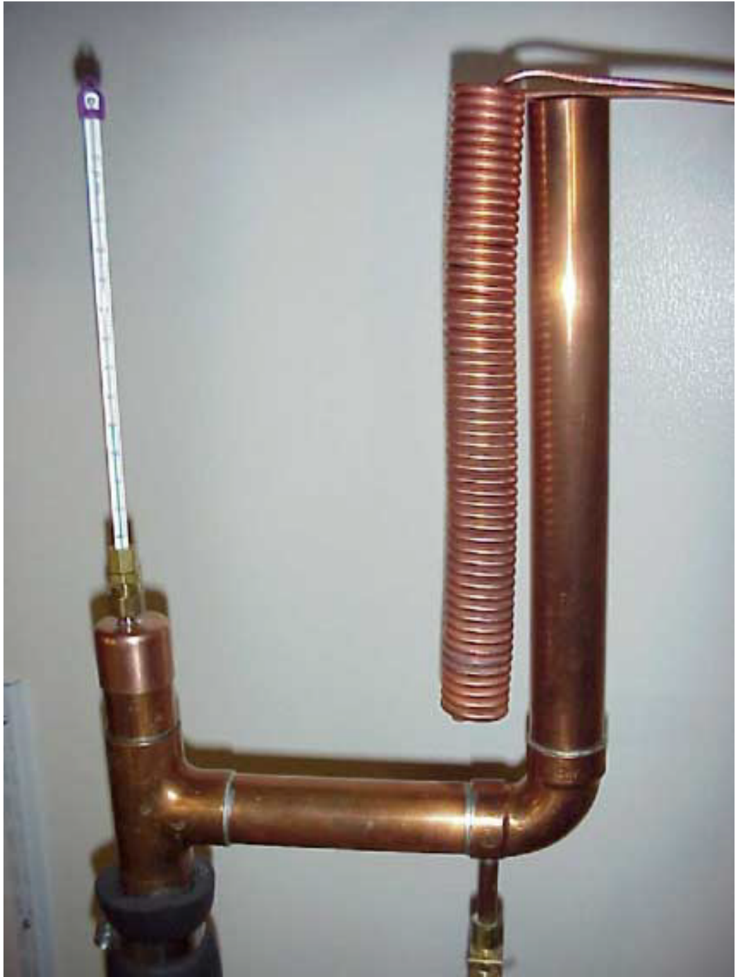
Still Head with Heat Exchanger Revealed
