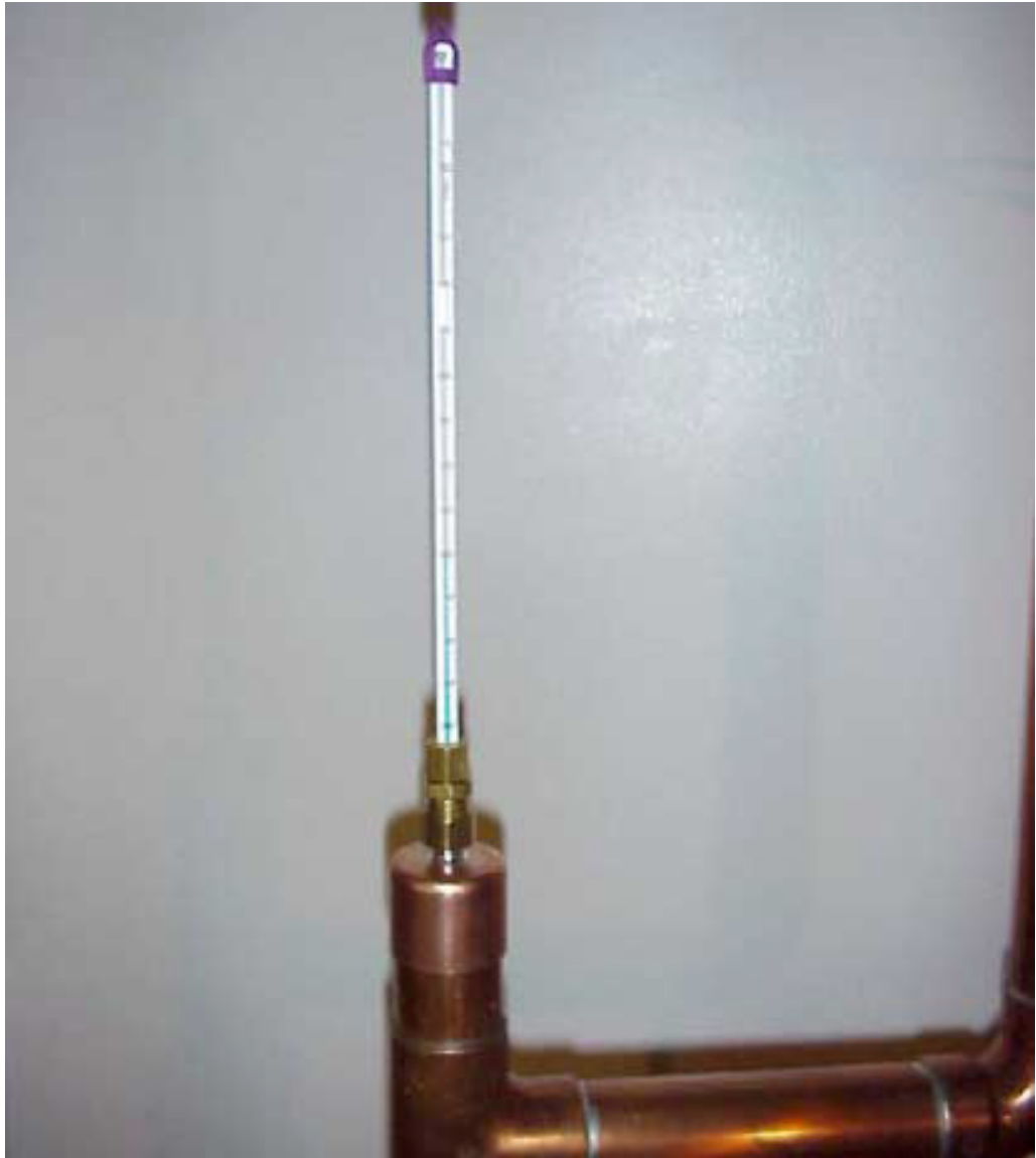
Thermometer Mounted with Compression Coupling
