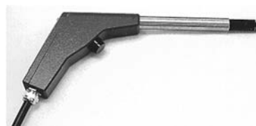
Figure 8. A commercial hand-held liquid probe for off-line or at-line analysis.
