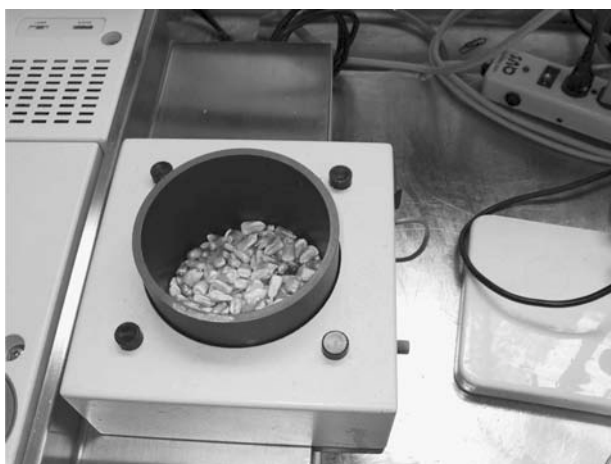
Figure 11. A rotating cup full of whole kernel corn on an integrating sphere.
