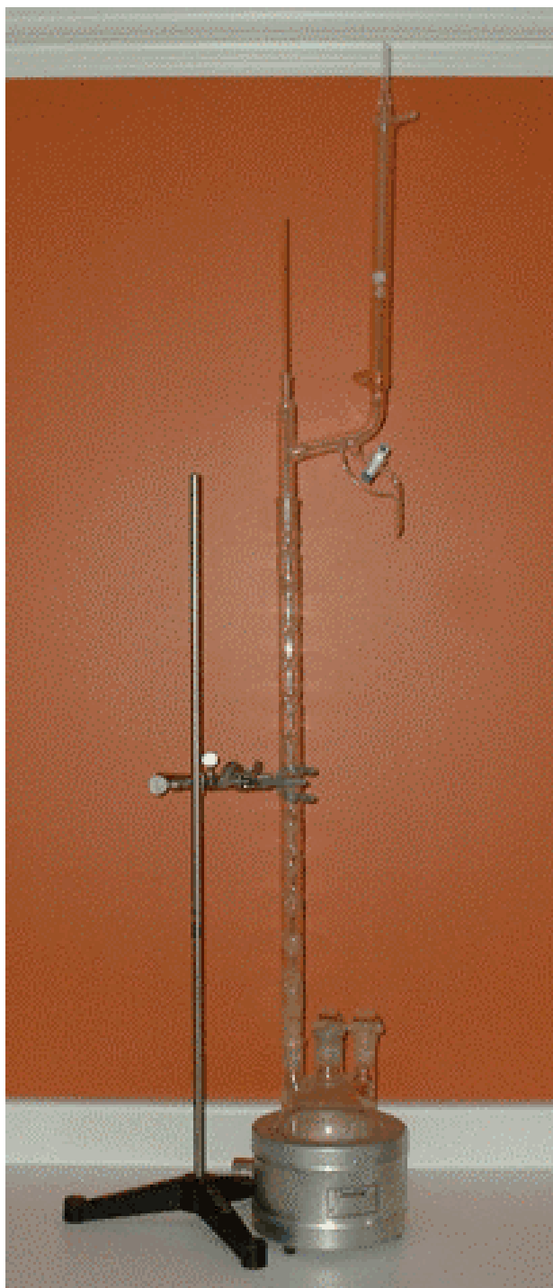
Figure 3. Laboratory fractionating still (Vigreux)
