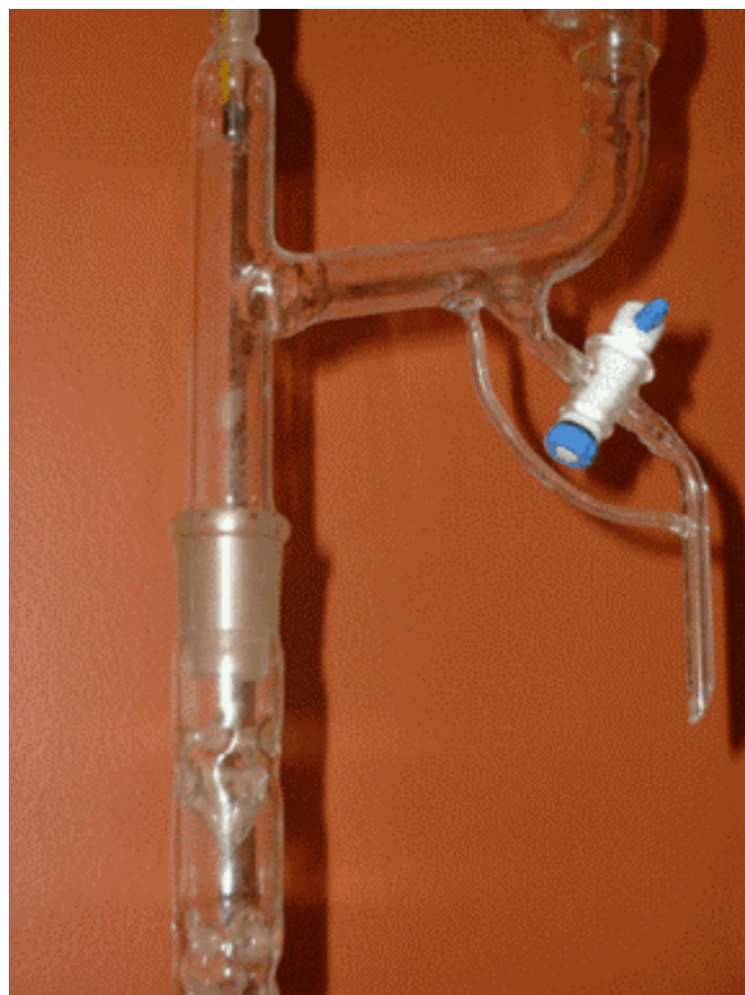
Figure 3. Laboratory fractionating still (Vigreux)
